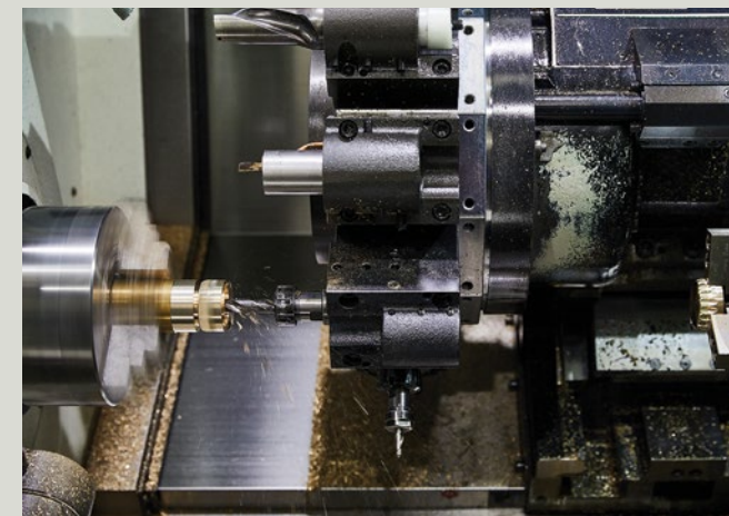
One of our sustainable production processes — brass shavings and swarf from manufacturing are recycled by being melted down into new brass components.
