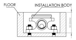
NB : ENSURE BODY IS INSTALLED AT CORRECT DEPTH 50 - 55MM BELOW FINISHED FLOOR
