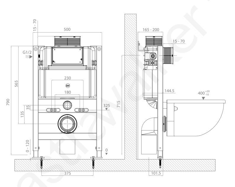
**NOTE**: There should be no gap between the wall & cistern frame. The wall should be made of noncompressible materials
