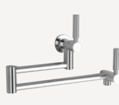
Pot Filler 534mm Reach from Wall 6 Star 4L/min WELS Rating
